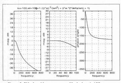
▲ Figure 6. PLL closed loop response with single pole LPF.
