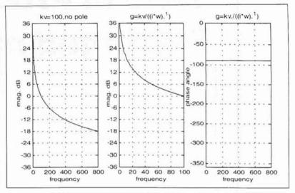
▲ Figure 2. PLL open loop transfer function with no loop filter.
