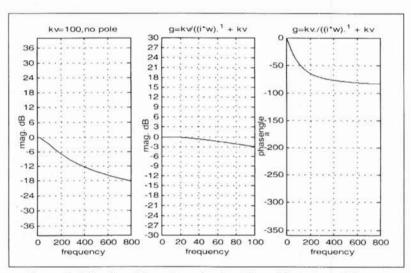
▲ Figure 3. PLL closed loop transfer function with no loop filter.
