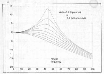
▲ Figure 7. Closed loop gain response vs. frequency for different damping factors (¬).
