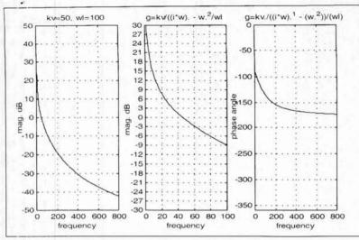
▲ Figure 5. PLL open loop response with single pole LPF.
