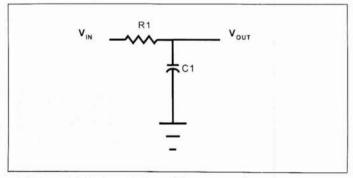
▲ Figure 4. Single pole loop filter.
